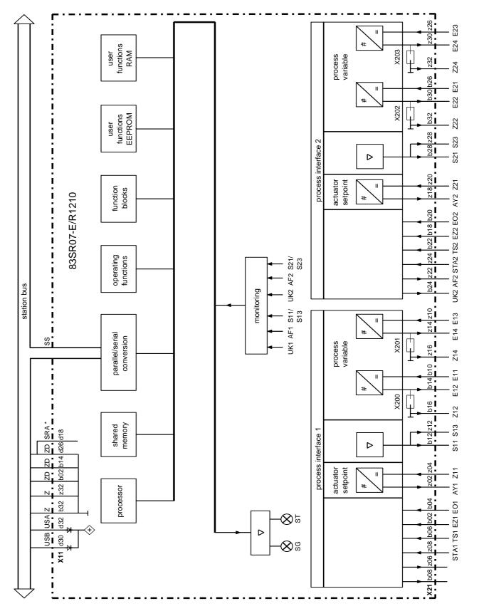
\* To ensure proper functioning of the module, terminal X11/d18 has to be connected with ZD (once per subrack).
