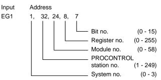
In the case of module inputs that receive their signals via the process interface, addressing is done by allocating the process interface to EGn. In this case, a distinction is to be made between contact inputs (VPn) and analog inputs (VAn), e.g.:
